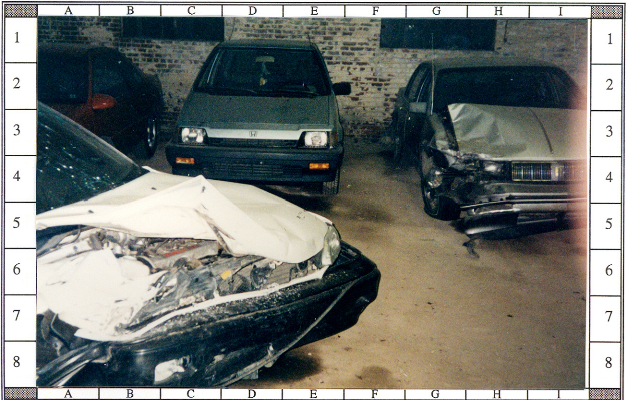
# 16: Vehicle #2's frontal crush viewed from right showing offset nature of crush profile, direct damage right fender, and induced damage to hood and windshield
